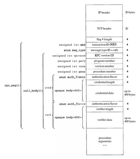
Figure 16.30 RPC request encapsulated in a TCP segment.
