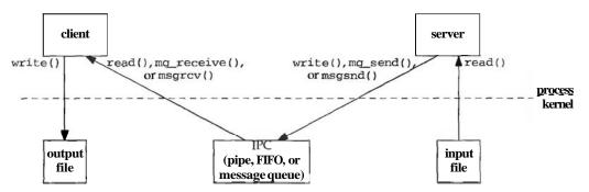
Figure 12.1 Flow of file data from server to client.
