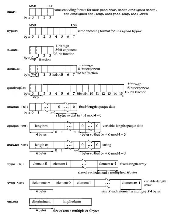
Figure 16.16 Encoding used by XDR for its various datatypes.
