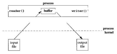
Figure 10.27 One process that reads data into a buffer and then writes the buffer out.
