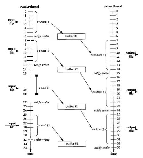
Figure 10.32 Time line for double buffering.
