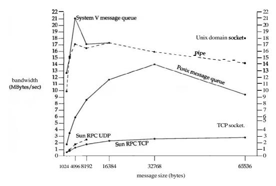
$\textbf{Figure A.5} \quad \text{Bandwidth for various types of message passing (Digital Unix \textbf{4.0B)}.}$
