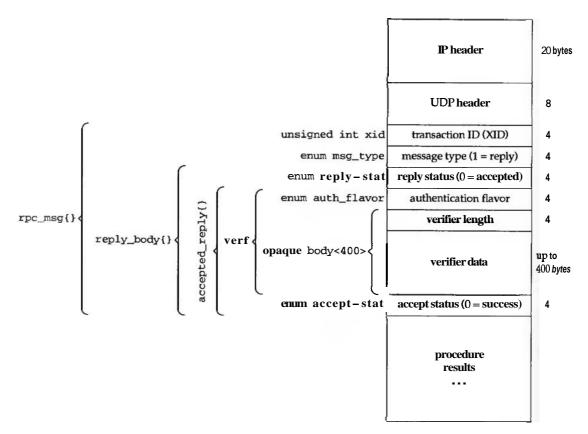
Figure 16.32 Successful RPC reply encapsulated as a UDP datagram.
