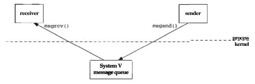
Figure D.7 Sending messages using a System V message queue.
