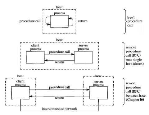
Figure 15.1 Three different types of procedure calls.
