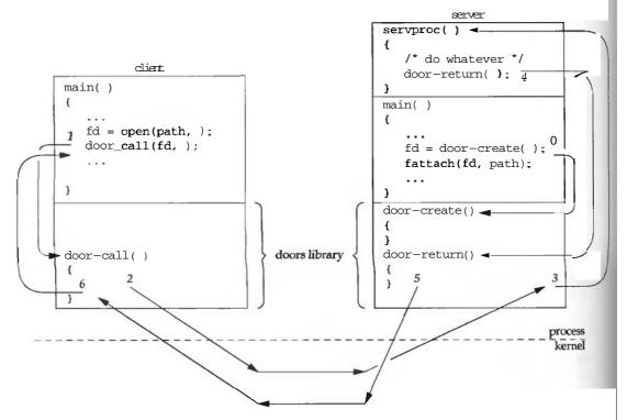
$\label{Figure 15.5} \textbf{ Actual flow of control for a procedure call from one process to another.}$
