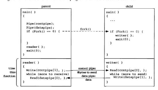
Figure A.14 Overview of program to measure the bandwidth of a pipe.
