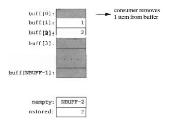
Figure 10.16 Buffer and semaphores after consumer removes first item from buffer.
